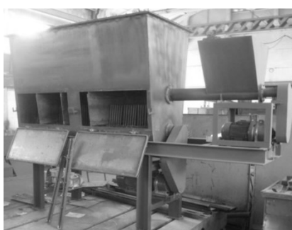
Fig. 2. General photo of the rotary drying unit with the possibility of drying fuel chips developed at the ITTF of the National Academy of Sciences of Ukraine.
