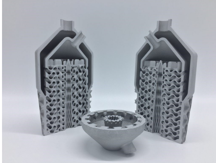
Fig. 1. Heat exchanger with gyroid canal [2]
